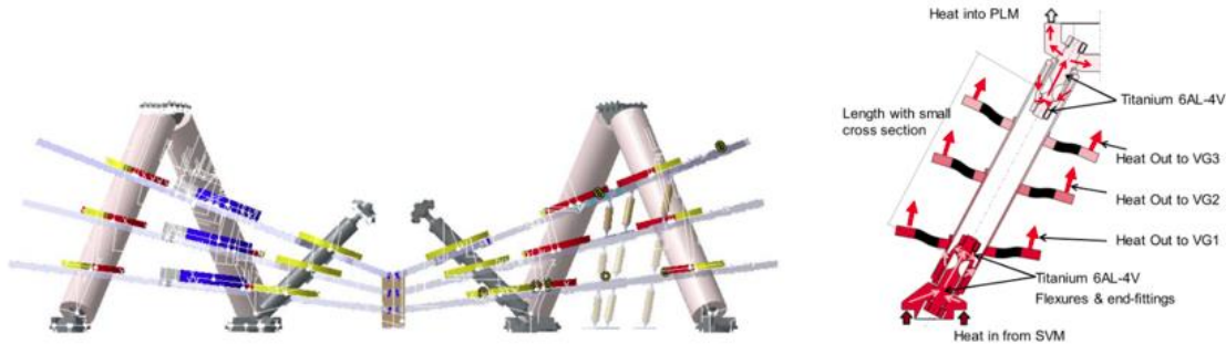
Figure 4. CFRP-made bipods and GFRP-made struts configuration as V-groove support (left); a bipod cross-section (right)
