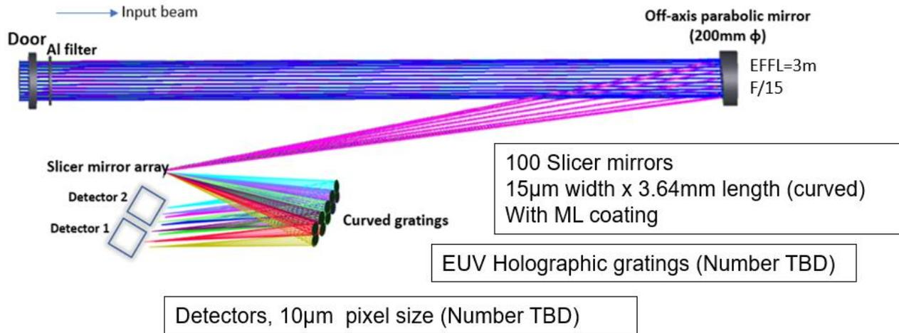
Figure 3. SISA conceptual optical design showing only ten configurations out of 100.
