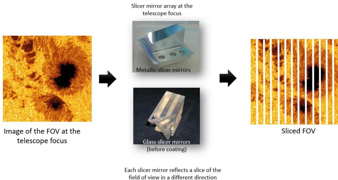
Figure 1. Sketch showing the concept of the sliced field of view (FOV) generated by the slicer mirror array at the telescope focus. The substrate for the slicer mirrors can be metal or glass as shown in this picture. In this example, the metallic slicer mirror array was manufactured at Durham University and the glass slicer mirror array, shown before depositing the coating, was manufactured by Winlight Optics, currently Bertin Winlight.
