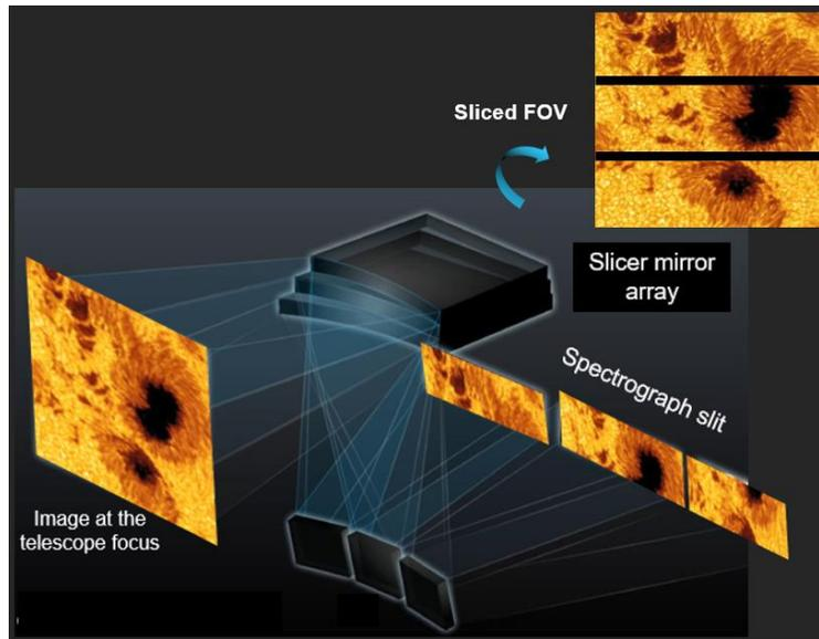
Figure 2. Sketch of an image slicer dividing the field of view in three slices to show the concept.
