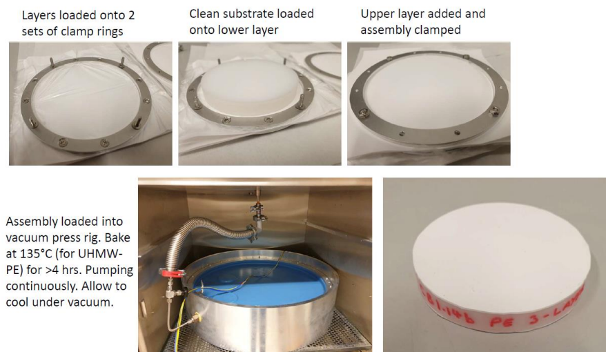
Figure 13. A view of the multi-layer ARC sample fabrication using the heat-bonding process.
