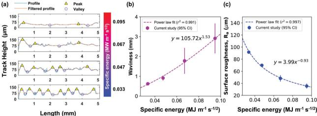
Figure 6. Topological analysis of Inconel 625 melt tracks as a function of specific energy (SE). a) The melt track profile, b) waviness ( $r^2 = 0.991$ , *p*-value = 0.00465), and c) surface roughness ( $r^2 = 0.997$ , *p*-value = 0.00167) plots as a function of SE.
