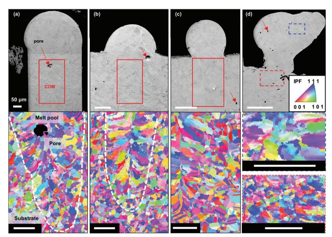
**Figure 7.** Backscattered electron images (BSEI) of Inconel 625 melt tracks processed at SE of a) 0.095, b) 0.067, c) 0.047, and d) 0.033 MJ m<sup>-1</sup> s<sup>-1/2</sup>. The red or blue region of interest indicates the corresponding crystal orientation map (COM) with an inverse pole figure (IPF) key. The white dotted lines show the interface between the melt pool and the substrate. Scale bar 50  $\mu$ m.
