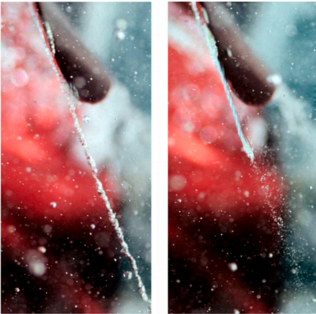
Fig. 4. Images of tip vortex cavitation from a propeller blade without thread (left) and with a flexible thread (right).
