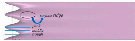
(b) Edge serrations on a foil. Reproduced from (Wang et al., 2021)
