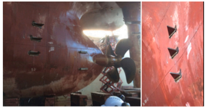
Fig. 3. Vortex generators fitted upstream of a propeller on a tanker. Source: Reproduced from Saydam et al. (2018) .
