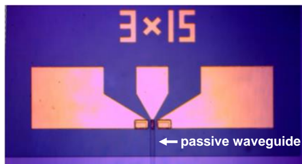
Figure 2.10: Fabricated 3x15 \mu\text{m}^2 CPW UTC-PD.
