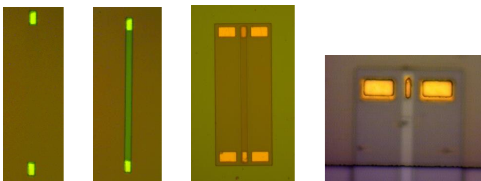
Figure B.2: From left to right: P-contact ridge etch, waveguide etch, mesa etch and vias etch.
