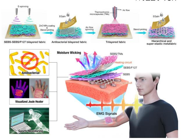
**Figure 1.** Schematic illustrating the fabrication of liquid metal printed hierarchical metafabrics with perspiration-wicking, visualized Joule heating, and antibacterial capabilities for advanced epidermal electrodes.
