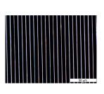
Figure 6. Optical microscope image taken with back illumination shows void apertures. It is important to note that etching of  $SiN_x$  by  $XeF_2$  is not efficient [39] and requires a separate processing step to remove it. Otherwise, the remaining  $SiN_x$  causes aperture widening defects: if a silicon nitride membrane gets broken in the one of the apertures, the tensile stress of the intact  $SiN_x$ membranes in the neighboring apertures pulls the gold bars
