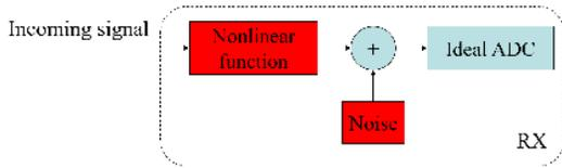
Fig. 1. A simplified model of a generic RX relevant to the scope of this work.
