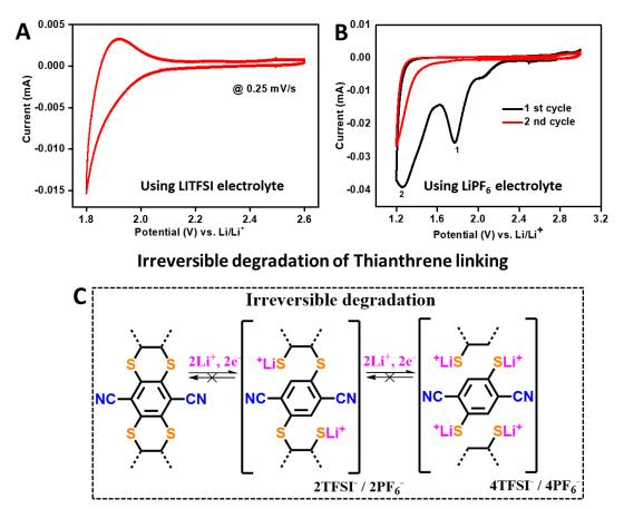
Figure S19. A. The CV of DUT-177 derived coin-cell using LiTFSI in DOL : DME (1:1) electrolyte (40  $\mu$ L). B. The CV of DUT-177 derived coin-cell using LiPF<sub>6</sub> in EC : DMC (1:1) electrolyte (40  $\mu$ L). C. Suggestion of a plausible pathway of irreversible degradation of dithine linkage upon Lithium interactions.
