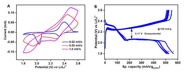
Figure S31: A. Cyclic voltammetry (CV) measurement at different scan rate of S-DUT-177 derived coin-cell in LiTFSI electrolyte. B. Charge-discharge profile of S-DUT-177 derived coin-cell at different current densities in LiTFSI electrolyte.
