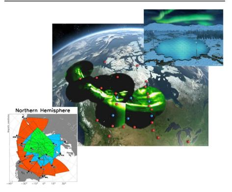
**Fig. 8** Schematics of a potential ground-based auroral addition to a magnetosphere-ionosphere coupling mission proposed here with (top right) EISCAT 3D and (bottom left) SuperDARN radar systems (adapted from http://vt.superdarn.org/)
