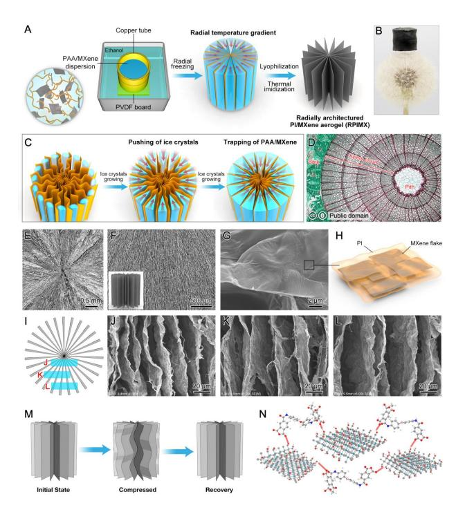
**Figure 1.** (A) Fabrication process of the radially architectured RPIMX composite aerogels. (B) The lightweight demonstration of the composite aerogel (it can stand steadily on a dandelion). (C) Illustration showing the formation of radiating structures using radial ice-templating strategy. (D) An optical microscope image showing the purple stained xylem tissue of *Liriodendron* stem
