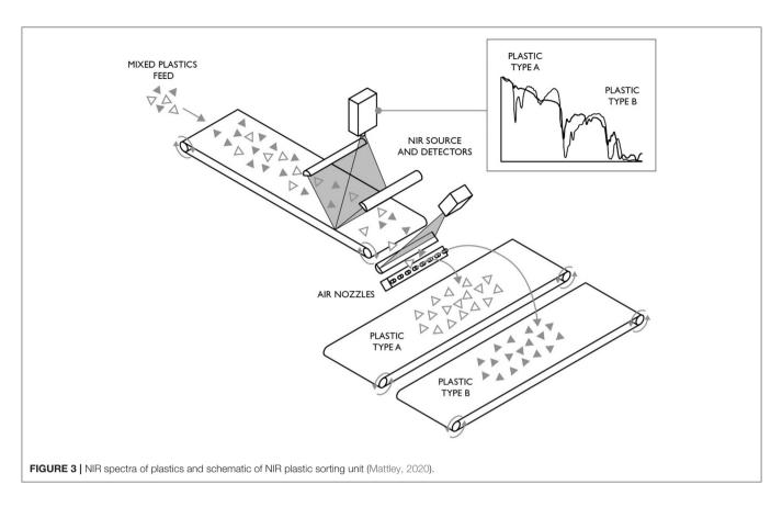
system consists of 3 main units which are the identification unit, the control unit and the throwing unit. When the plastics pass through optical sensors, they are determined by the identification unit and control unit. The target polymers are ejected from the plastic stream by ejection nozzles in the throwing unit. Parameters such the presence of labels, caps, thickness and surface contamination and color have been shown to affect the sorting efficiency of the system.
