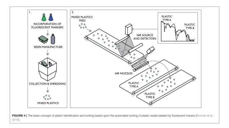
when adding additional fluorescent markers (Kosior et al., 2015). The lowest marker concentration is essentially defined by the ability of the measurement system to acquire fluorescence emission spectra with a signal-to-noise ratio (SNR) large enough to reliably perform the classification task. In case of black plastics which absorbs large part of the fluorescent light from the markers, a marker concentration (up to ~100 ppm) is needed (Brunner et al., 2015).
