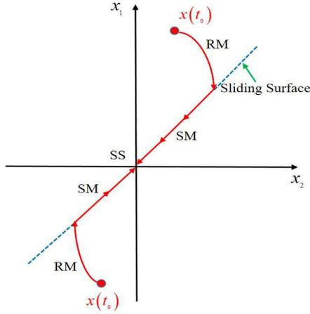
Fig. 1: Phase diagram of continuous SMC.
