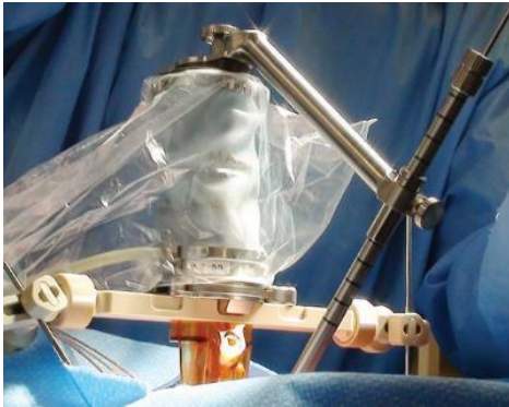
Fig. 10. The Renaissance system is a passive patient mounted parallel robotic manipulator designed to assist in the placement of spinal pedicle screws [4].
