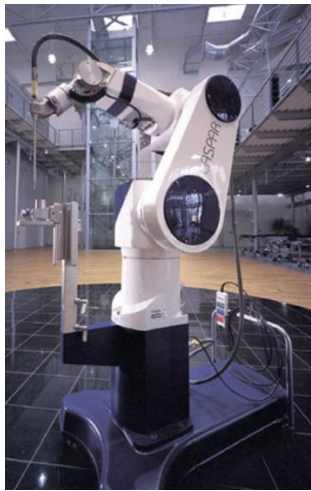
Fig. 3. CASPAR was an active surgical robot system designed to optimize outcomes in orthopedic surgical procedures [112].
