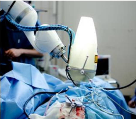
Fig. 13. The CARLO robotic system utilizes laser technology for ablation and cutting of bone [115].
