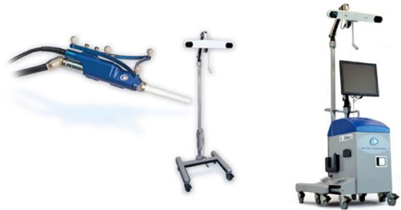
Fig. 8. The Navio PFS is a handheld semi-active robotic system [111] used in partial and total knee arthroplasty procedures.
