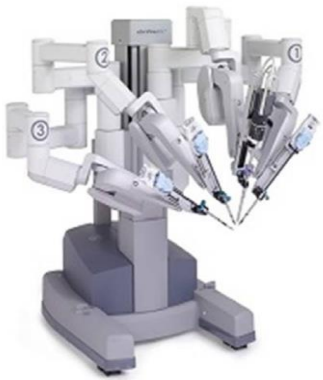
Fig. 2. The DaVinci can be classified as a tele-manipulator system in which direct input motion from the surgeon is filtered and scaled. It is widely used in soft tissue surgery in a number of fields [111].
