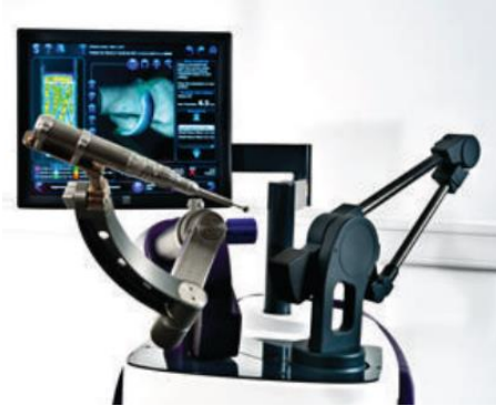
Fig. 4. The semi-active Acrobot system designed for partial and total knee arthroplasty procedures [4].
