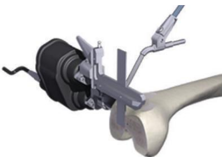
Fig. 7. The iBlock system is a passive, bone-mounted robotic cutting guide used in total knee arthroplasty procedures [4].
