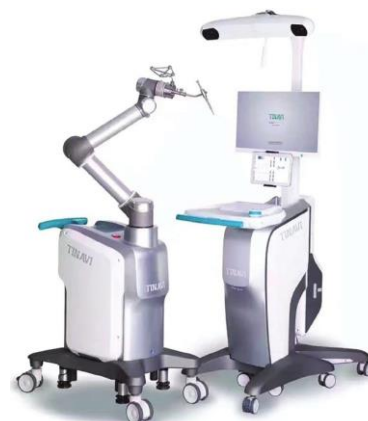
Fig. 9. The Tinavi system is a passive robotic arm designed to assist with spinal and pelvic surgeries [117].
