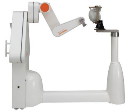
Fig. 11. The passive surgical robot Neuromate is designed for assistance during neurosurgical interventions [4].
