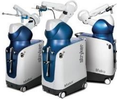
Fig. 6. The Stryker MAKO system is widely used for partial and total knee, as well as total hip, arthroplasty procedures. It functions in a semi-active control mode [113].
