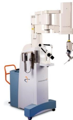
Fig. 5. ROBODOC is an autonomous surgical robotic system for hip and knee arthroplasty [27].
