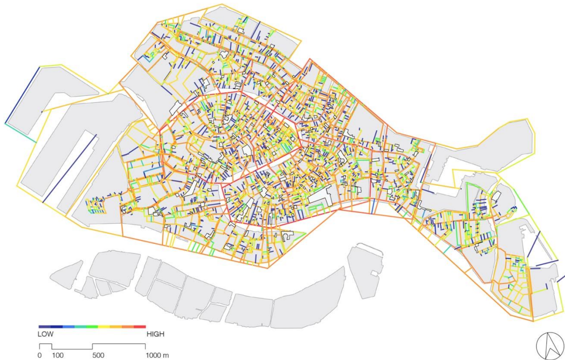
Figure 2. Betweenness centrality of combined pedestrian and canal networks, Venice (3b) – Drawing by Sophia Psarra, in (2018) The Venice Variations: Tracing the Architectural Imagination , UCL Press
