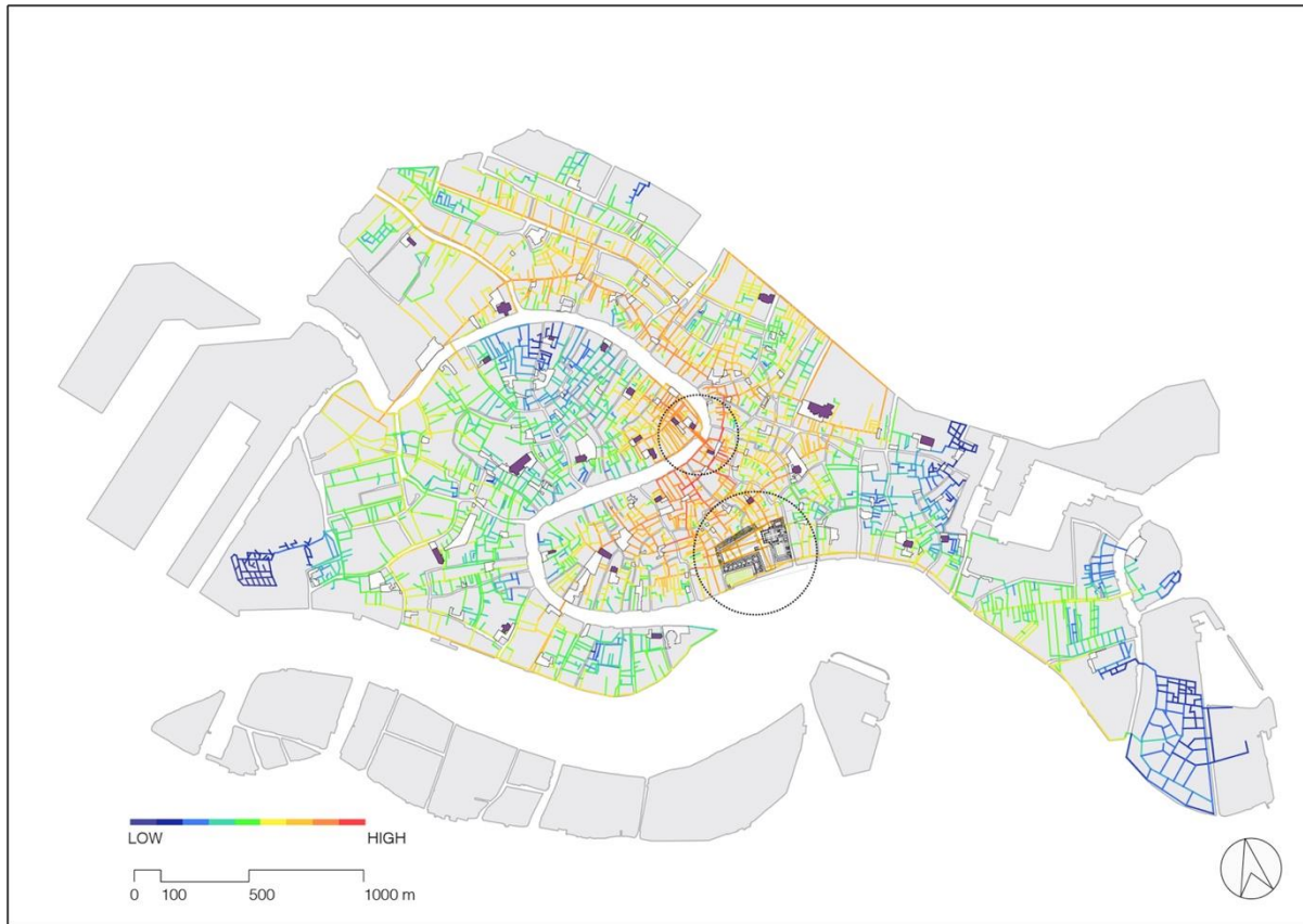
Figure 4 Closeness centrality values (Integration) of pedestrian network in Venice. Integrated spaces are easy to reach from every other space in a layout, constituting the spaces of where movement paths converge. In contrast, segregated spaces can be accessed through paths that involve many changes in direction. Drawing by Sophia Psarra, in (2018) The Venice Variations: Tracing the Architectural Imagination , UCL Press.
