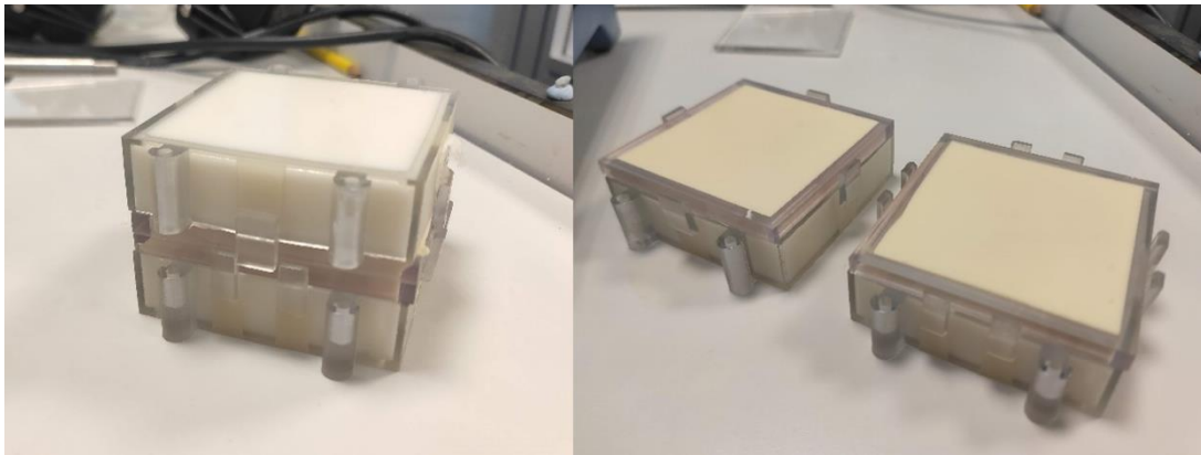
Figure 5-5. The 4-layered phantom. Left, the four layers stacked onto each other. Right, the phantom split in half, showing the central surfaces of the phantom.
