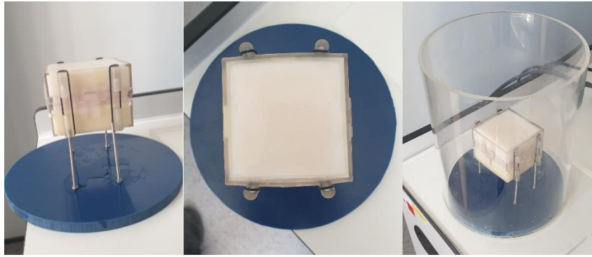
Figure 5-16: The phantom mounted atop the platform. Left, side view. Centre, top view. Right, The platform inside the tank.
