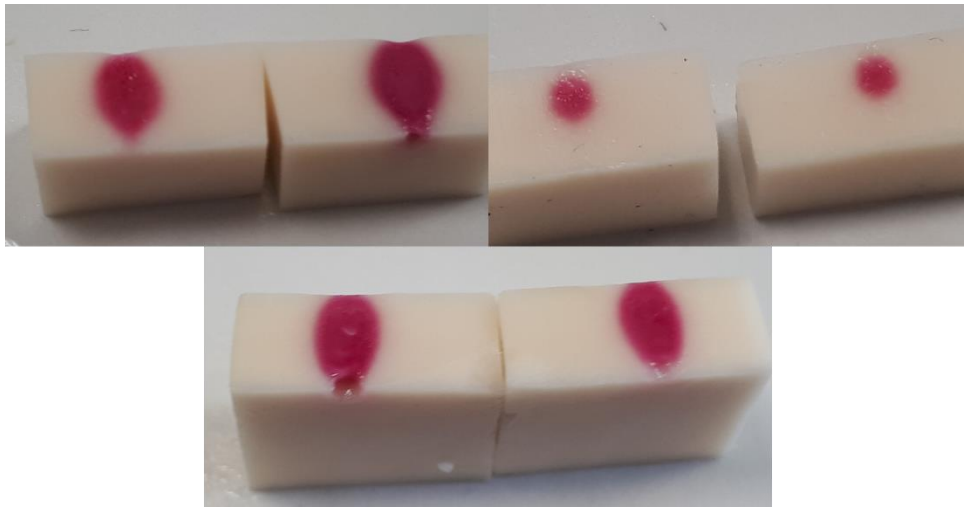
Figure 6-5. 158.5 p-p mV MPa exposures on the thermochromic slabs. From first to last: top left, top right, bottom.
