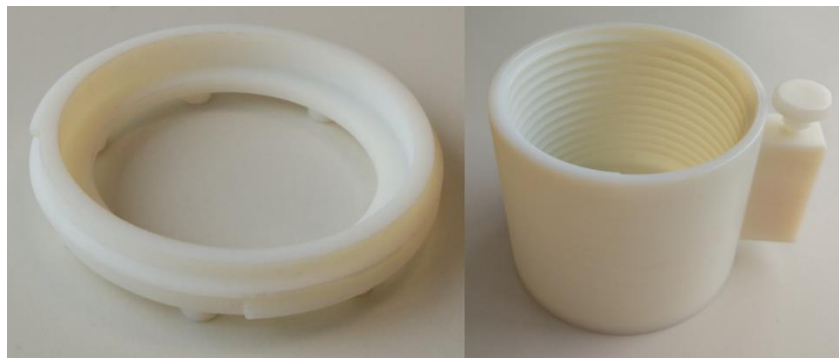
Figure 3-5: Adjustable, membrane-less solid sample holder. Left, the lid, Right, the body.
