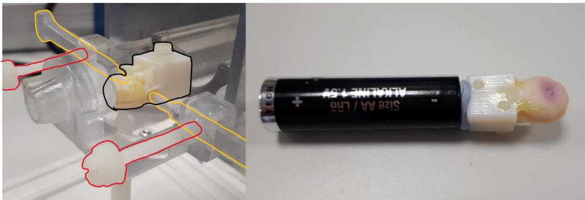
Figure 6-4: Left, the rods being used to hold the skull phantom in place. The rods, marked by the yellow outlines, were inserted into the ocular cavities of the skull phantom, marked by the black outline. Plastic screws, marked by red outlines, affix the position of the rods. Right, a battery was attached to the phantom so it could rest on the bed for better stability.
