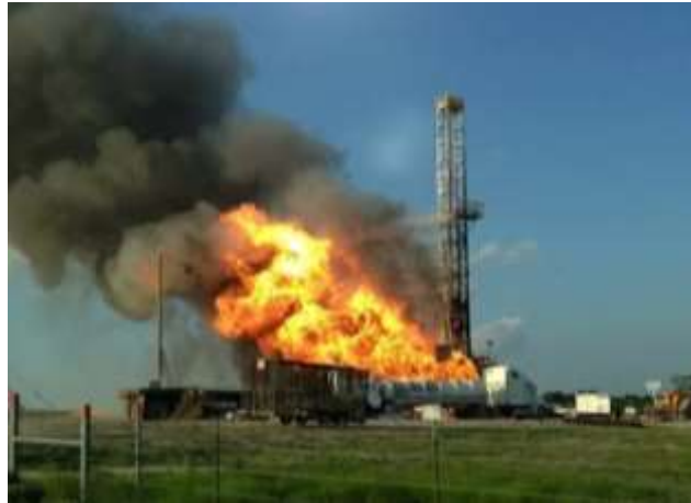
Figure 1. A blowout from a well drilled into Eagle Ford shale in Texas 10 .
