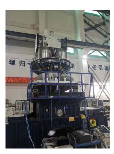
Fig. 11 Satellite STM on the shaker
