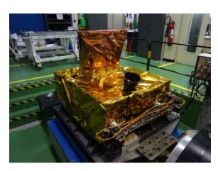
Fig. 9 PLM STM on shaker in ESTEC
