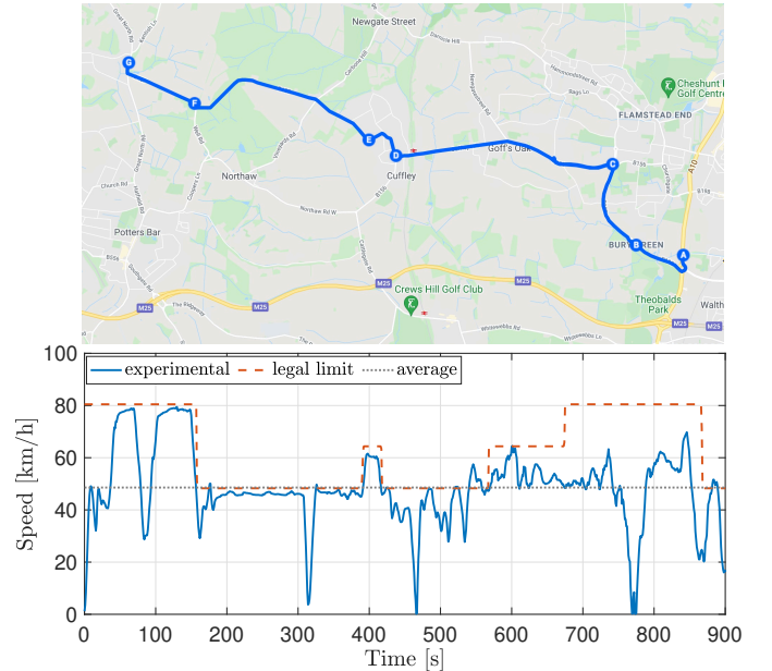
Fig. 11. Top: 12.1km rural route selected as a real-world vehicle driving mission https://t.ly/n2wL . Bottom: Experimental driving speed profile for the mission above.
