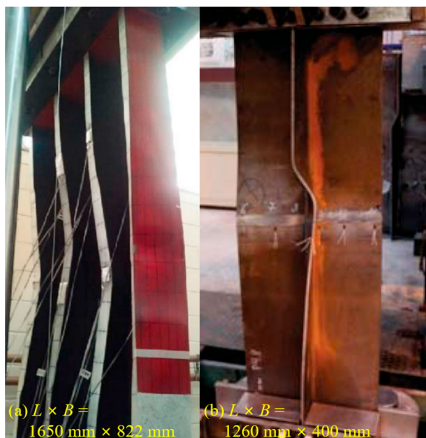
Figure 8. Deformed stiffened panels after collapse testing (2/2) (a) Manco et al. (2019), (b) Woloszyk et al. (2020).
