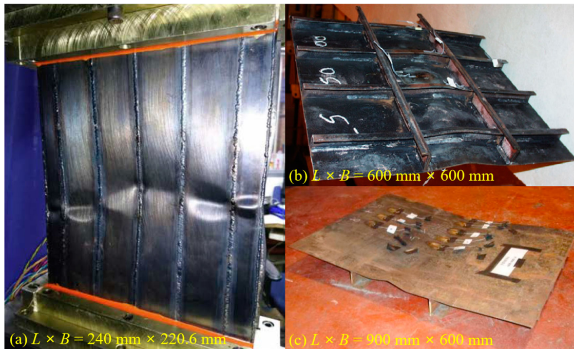
Figure 7. Deformed stiffened panels after collapse tests (1/2) (a) Chujutalli et al. (2020), (b) Gordo and Guedes Soares (2008), (c) Xu and Guedes Soares (2021).
