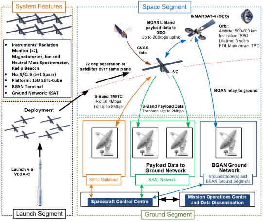
Figure 6-4: Mission Architecture 2 Concept of Operations (CONOPs)
