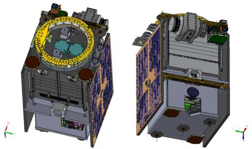
Figure 6-2: SSTL-21 D3S Spacecraft Concept in the Stowed Configuration
