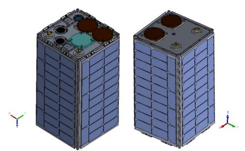
Figure 6-5: 16U SSTL-Cube D3S Spacecraft Concept in the Stowed Configuration
