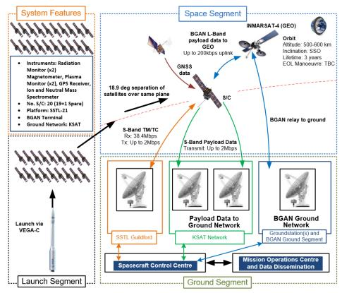
Figure 6-1: Mission Architecture 1 Concept of Operations (CONOPs)
