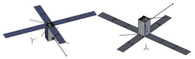
Figure 6-6: 16U SSTL-Cube D3S Spacecraft Concept in the Deployed Configuration
