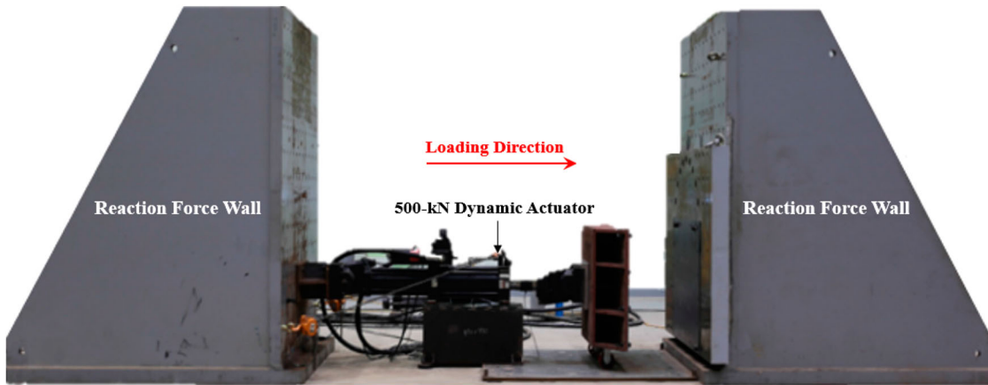
Figure 8. Photograph of the pneumatic rubber fender crushing test equipment.
