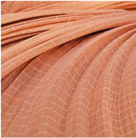
Figure 5. Synthetic tyre cord fabrics forming the middle layer that reinforces the pneumatic rubber fender.
