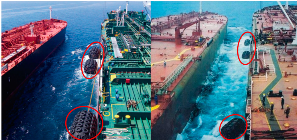
Figure 2. Pneumatic rubber fenders (red ellipses) for absorbing and dampening the impact energy during side-by-side collisions between a ship-shaped offshore installation and a shuttle tanker.
