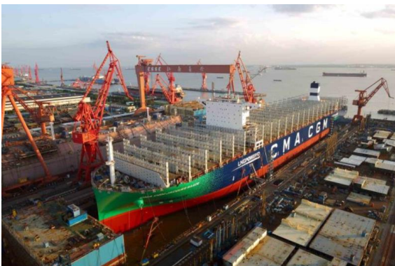
Fig. 2. A 23,000 TEU LNG-fuelled containership under construction (Swift, 2019).
