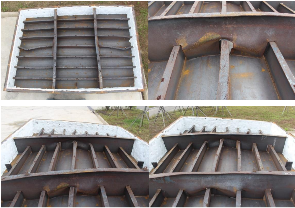
Figure 3.37 Deformed shapes of the test structure for the fire test without PFP.
