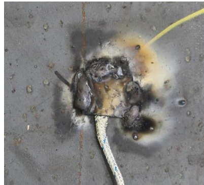
Figure 3.27 Spot welding to attach thermo-electric couple sensors.
