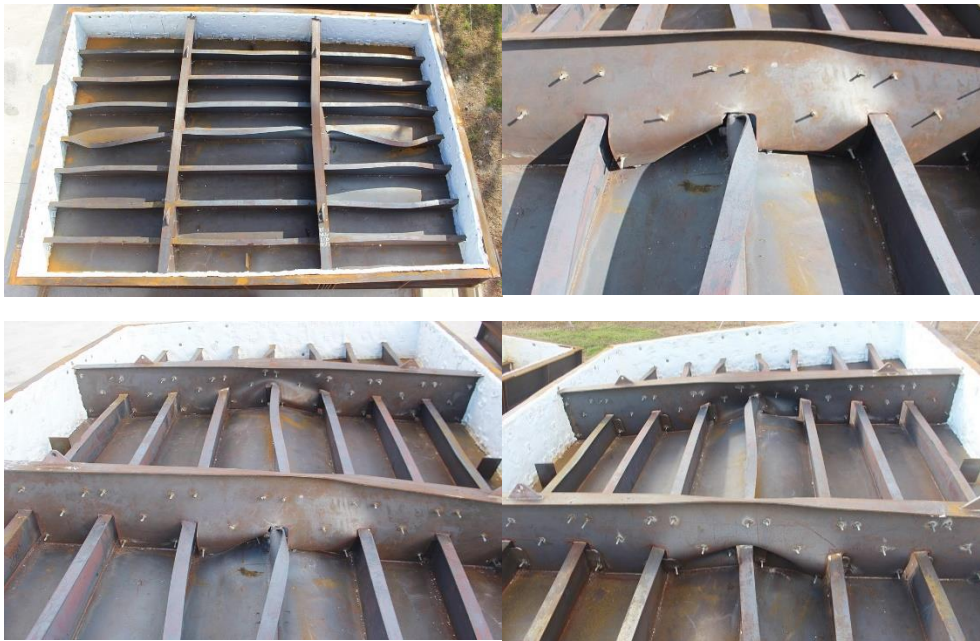
Figure 3.43 Deformed shapes of the test structure for the fire test with PFP (fire protection materials were removed).
