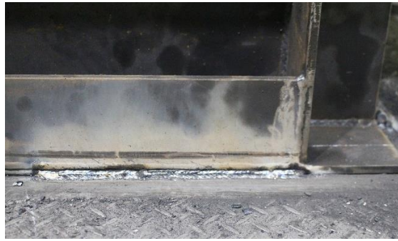
Figure 3.14 A 300 mm long welding of a supporting jig along part of the furnace boundary.
