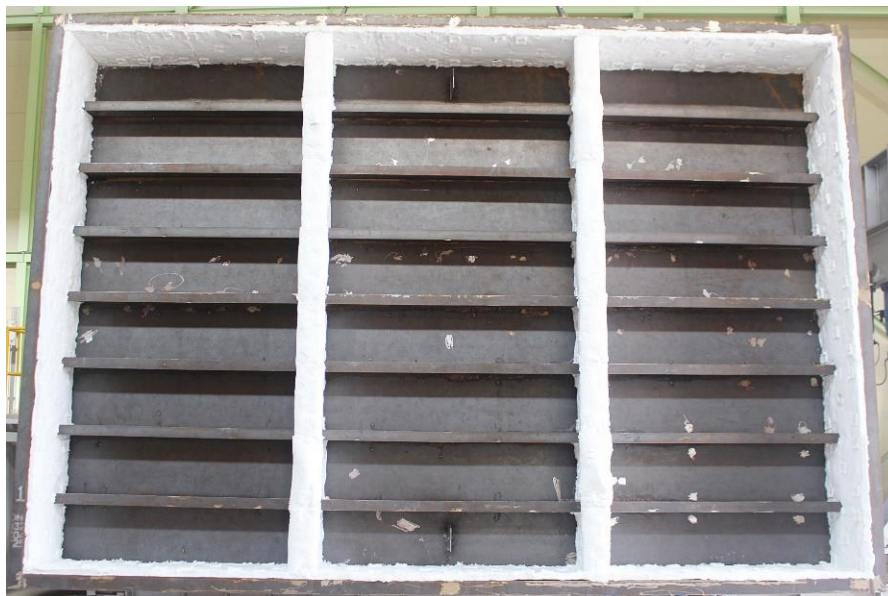
Figure 3.17 Insulation with passive fire protection material along the four boundaries and two transverse frames of the test structure for the fire test with PFP.
