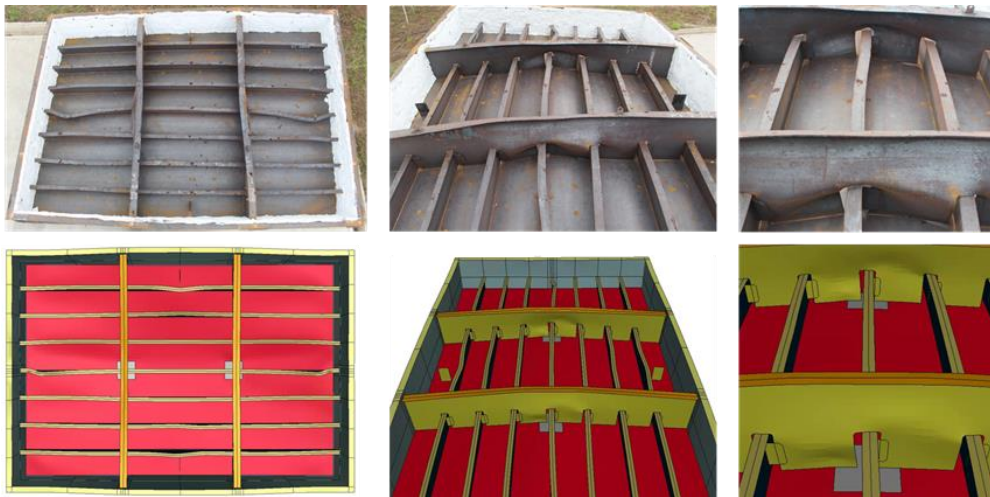
Figure 4.11. Comparison of the deformed shape for the structure without PFP after the collapse between the tested structure and the computation.
