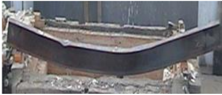
Figure 2.10 Deformed shape of the beam at collapse state obtained in the experiment (Cong et al. 2005).
