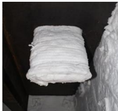
Figure 3.30 The sensor No.22 with fire protection using cerawool.
