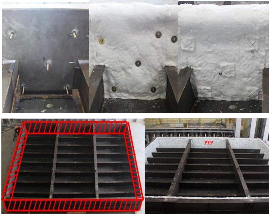
Figure 3.16 Insulation with passive fire protection material along the four boundaries of the test structure for the fire test without PFP.
