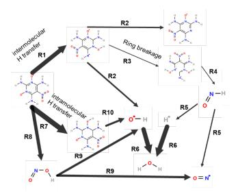
**Figure 5.** Primary reaction pathways for the ICM-102 decomposition and formation of H<sub>2</sub>O. The arrow width represents the observed number of reactions (n), where width =  $\ln (n+1)$ .
