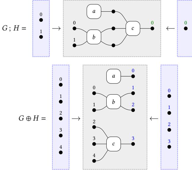
The composition and tensor product in  $\text{Csp}_D(\text{Hyp}_\Sigma)$  now give us a way to interpret string diagrams (or more precisely,  $\Sigma$ -terms) as hypergraphs. For each of the generators  $o : m \rightarrow n$  in  $\Sigma$ , we can form a cospan  $m \rightarrow O \leftarrow n$  where  $O$  consists of a single  $o$ -labelled hyperedge with  $m$  input nodes and  $n$  output nodes
