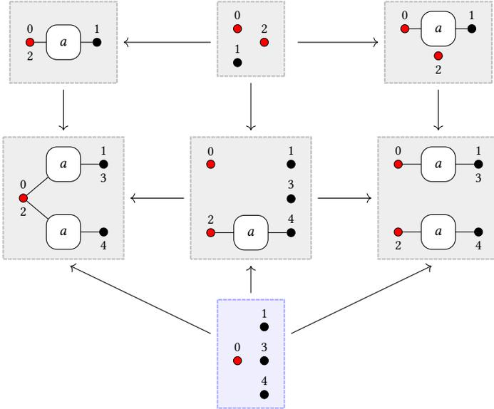
Note that the node labelled 2 in the resulting graph is not in the image of the interface (corresponding to a ) and the node labelled by 1 and 3 is in the image of two nodes in the interface (corresponding to a ). Hence, the outcomes of syntactic and DPOI rewriting coincide.
