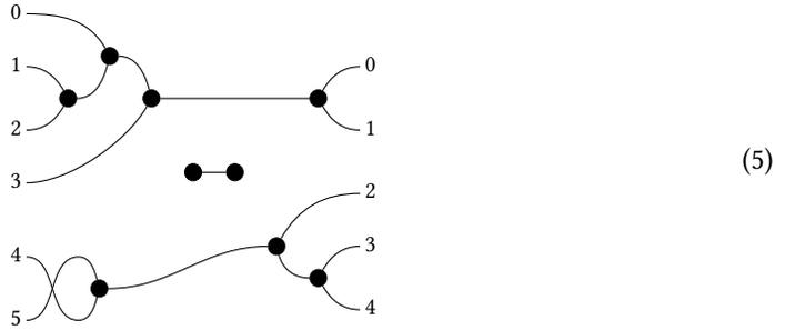
To represent a morphism in  $\mathbf{Frob}$  as a cospan, the inputs become the set on the left, the outputs the set on the right, and the connected components of generators in the diagram form the middle set. The two functions in the cospan then respectively map each input or output to its associated connected component
