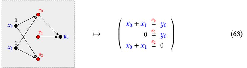
This interpretation gives a semantical view of the **Reduction Strategy** as a quantifier elimination procedure. The main purpose of the procedure is to eliminate interior  $\bullet$  nodes. Since these nodes arise from sequential compositions in  $\mathbf{LinRel}(\mathbb{Z}_2)$ , equation (62) tells that they correspond to existentially quantified variables
