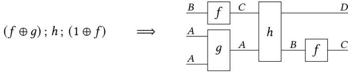
The relevant data of such a composition is the connectivity, rather than the physical layout of the boxes and wires. Hence, it makes sense to consider ‘crossing’ of wires, and the SMC axioms make the interpretation invariant under deformation, e.g.
