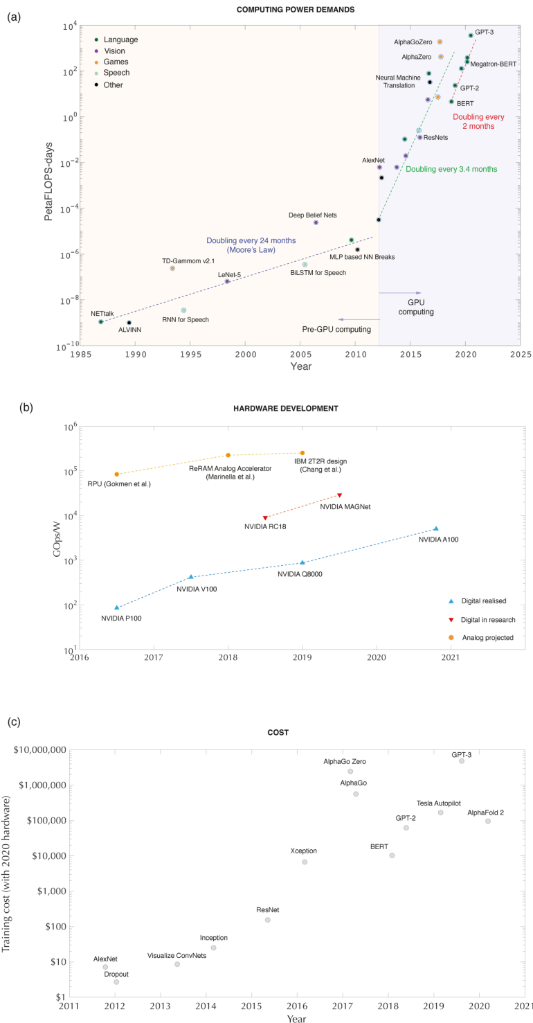
Figure 1. Computational demands are increasing rapidly. (a) The increase in computing power demands over the past four decades expressed in PetaFLOPS-days. Until 2012, computing power demand doubled every 24 months; recently this has shortened to approximately every two months. The colour legend indicates different application domains. Data taken from [3]. (b) Improvements in AI hardware efficiency over the last five years. State-
