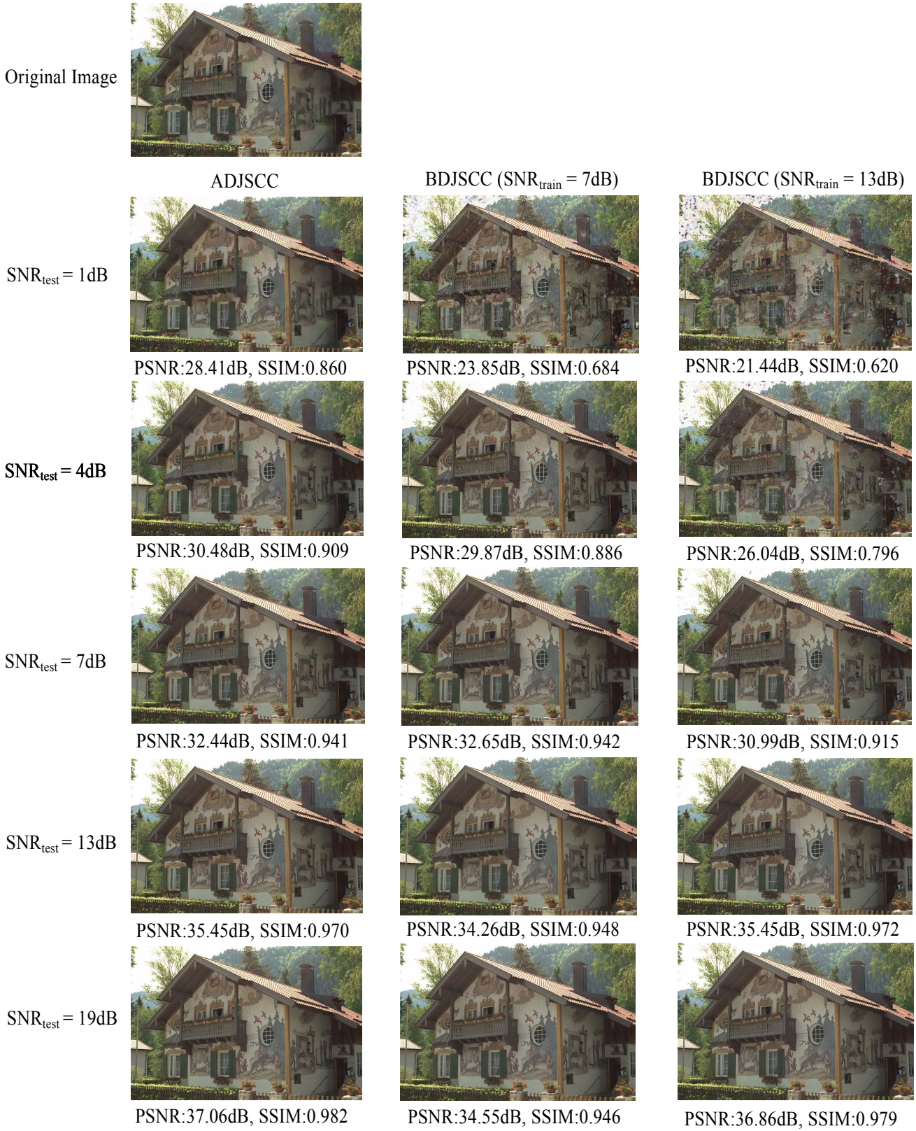
Fig. 11. Visual comparison between the ADJSCC model and the BDJSCC models (SNR train = 7dB, 13dB) for the sample image of the Kodak dataset. We also used a perceptual metric—structural similarity index (SSIM)—to evaluate image quality.
