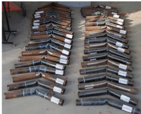
Fig. 1. Rehabilitation of corroded steel pipelines specimens [10]
