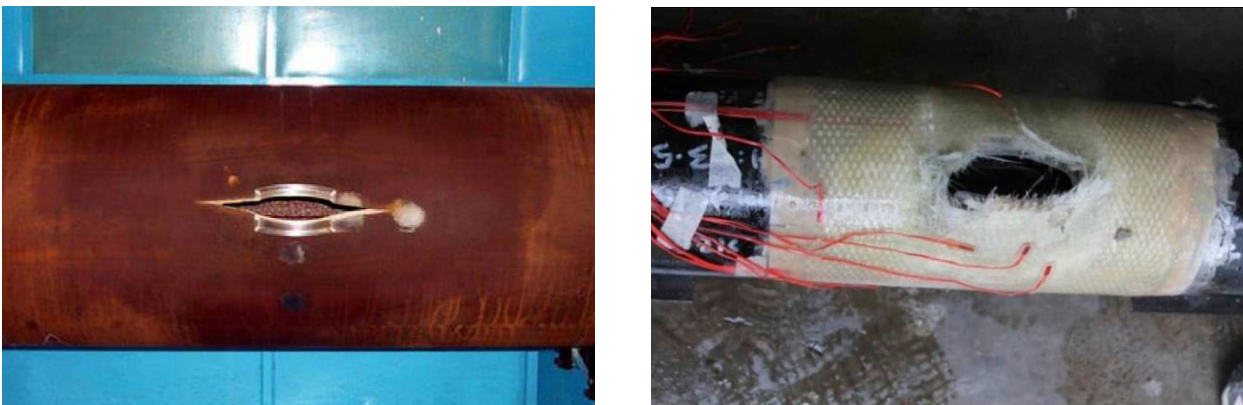
Fig. 7. Pipelines burst pressure test based on past studies by (left) [22] and (right) [5] for the validation of the pilot FE model
