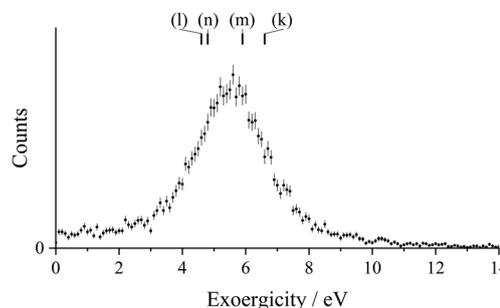
Fig. 10 Experimental exoergicities spectrum for the reaction  $S^{2+} + N_2 \rightarrow S^+ + N_2^+$ . The error bars represent two standard deviations of the associated counts. The literature exoergicities resulting from the pathways (k)–(n) are indicated. See text for details.
