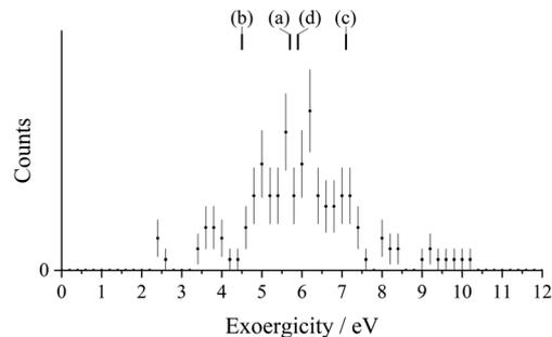
Fig. 2 Experimental exoergicity spectrum for the reaction  $\text{S}^{2+} + \text{Ar} \rightarrow \text{S}^+ + \text{Ar}^+$ . Calculated literature exoergicities for the potential SET pathways are also shown (pathways (a)–(d), discussed in the text). The error bars represent two standard deviations of the associated counts.
