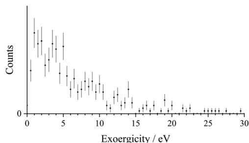
Fig. 7 Experimental exoergicity spectrum for the dissociation of  $\text{H}_2^+$  to form  $\text{H}^+ + \text{H}$ . The  $\text{H}_2^+$  is formed *via* the initial electron-transfer reaction  $\text{S}^{2+} + \text{H}_2 \rightarrow \text{S}^+ + \text{H}_2^{+*}$ . The error bars represent two standard deviations of the counts. See text for details.
