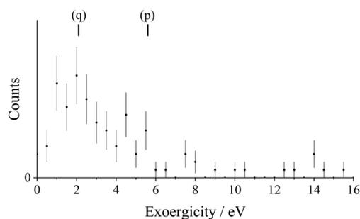
Fig. 13 Experimental exoergic spectrum for the reaction  $S^{2+} + N_2 \rightarrow SN^+ + N^+$ . The error bars represent two standard deviations of the associated counts. The literature exoergicities of potential reaction pathways (p) and (q) are indicated. See text for details.
