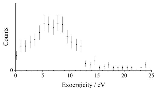
Fig. 8 Experimental exoergicity spectrum determined from precursor velocities for the initial electron-transfer reaction in the DSET channel,  $\text{S}^{2+} + \text{H}_2 \rightarrow \text{S}^+ + \text{H}_2^{+*} [\rightarrow \text{S}^+ + \text{H}^+ + \text{H}]$ . The error bars represent two standard deviations of the associated counts. See text for details.
