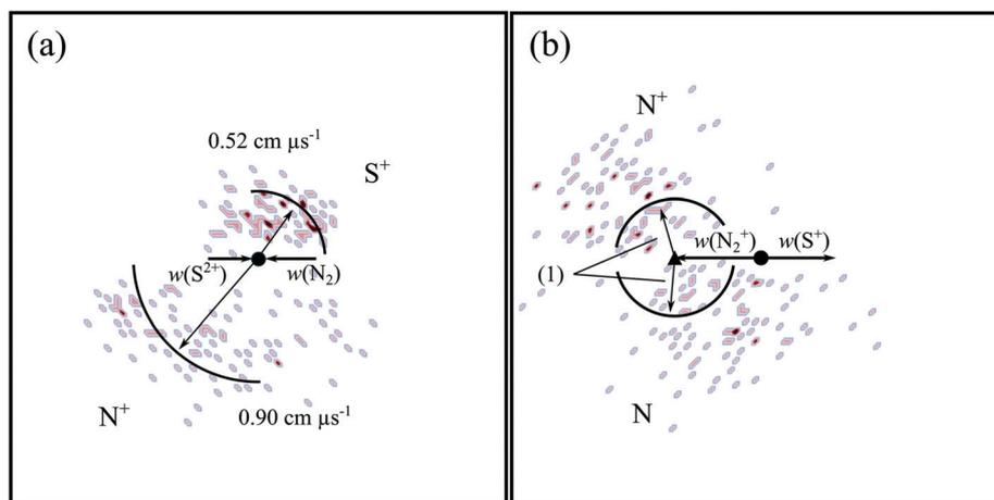
Fig. 11 Scattering diagrams for the DSET reaction  $S^{2+} + N_2 \rightarrow S^+ + N^+ + N$  at a CM collision energy of 4.7 eV. The black dot indicates the position of the CM. (a) CM scattering diagram showing the  $S^+$  and  $N^+$  products relative to the incident dication velocity,  $w(S^{2+})$ . (b) Internal frame scattering diagram showing the scattering of  $N^+$  and  $N$  relative to  $w(S^+)$ . In part (b) the labelled vector, (1), represents  $0.44 \text{ cm } \mu\text{s}^{-1}$ .
