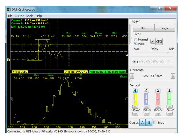
Figure 6-8 DRS Oscilloscope software screen capture
