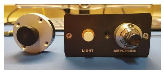
Figure 6-14 SP5601 LED driver (right) and the DS2628 sensor holder (left)
