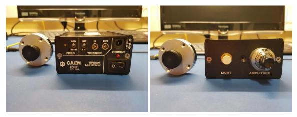
Figure 6-2 SP5601 LED driver with the SP5650 sensor holder (the round piece on the left). The left is the back of the SP5601 and the right is the front.
