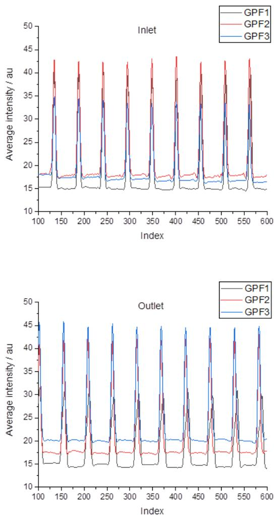
Figure 6: (Top) Inlet and (Bottom) outlet average intensity in the plug regions over a 3.2 mm depth, 20x20 mm sub-volume.
