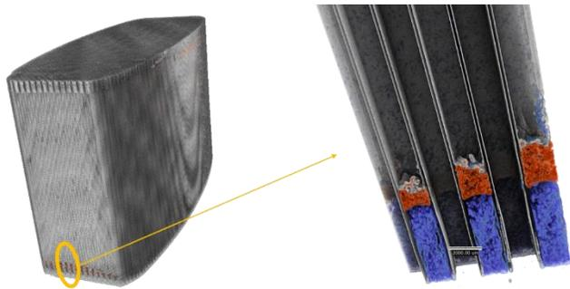
Figure 2:  $\mu$ -CT rendering of GPF 2, highlighting the channel walls (grey) channel plugs (blue) and iron oxide ash (red). Left hand side is 70.3  $\mu$ m overview, right hand side is close up from 32.1  $\mu$ m ROI scan.
