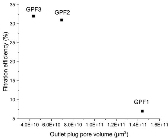
**Figure 10:** (Top) Correlation between average channel width and backpressure; (Bottom) Correlation of final filtration efficiency with outlet plug pore volume (operating point 1). Values are total areas/volumes summed over 200 complete channels/plugs.
