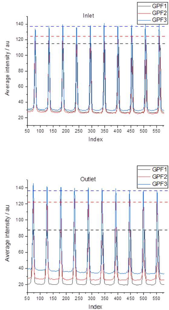
Figure 5: (Top) Inlet and (Bottom) outlet average channel intensity over a 16 mm depth, 20 x 20 mm sub-volume. The dashed horizontal lines are included to aid comparison of the average intensity for the channel walls along view direction for each filter inlet/outlet. The average intensity of the channel walls across the view direction are visible in the troughs between peaks.
