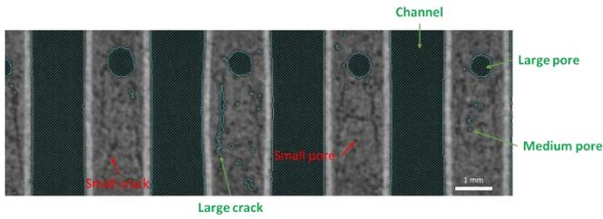
**Figure 9:** Example of segmentation of pores and cracks within plug regions highlighting the features that could (green) and could not (red) be reliably segmented.
