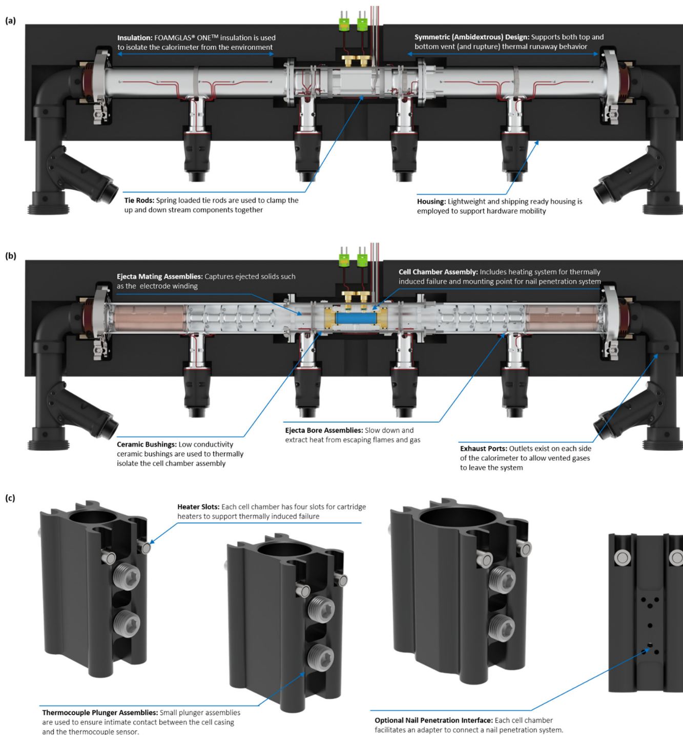
Fig 1 Rendered images of the fractional thermal runaway calorimeter (FTRC) where (a) identifies the fractional calorimeter exterior with the housing and FOAMGLAS® ONE™ insulation, the tie rod assemblies, and the symmetric design highlighted, (b) uses a cutaway view to highlight the primary FTRC sub-assemblies, ceramic bushings, and exhaust ports, and where (c) depicts the three different cell chambers (i.e. 18650, 21700, and D-Cell) and their key features. Note that the device as depicted with (a) and (b) is ambidextrous to support cells with both top and bottom vents where bottom vent cells can experience rupture from both ends of the cell; this design also accommodates top vent cells experiencing a breach at the bottom of the cell.
