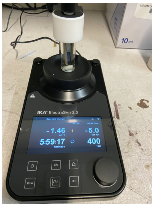
Figure 44: Image of an IKA Electrasyn set up for a constant current electrosynthetic oxytrifluoromethylation reaction of styrene using trifluoroacetylpyridinium.
