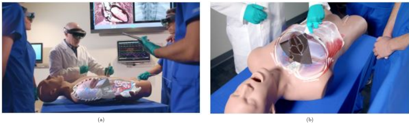
Fig. 12: Surgical Training Example Application: Ultrasound Education. (a) Multiple users can see holographic anatomical cross sections mapped on a patient simulator and the ultrasound scan plane. (b) Holographic subcostal four-chamber view coming out of the simulator probe. Source: Fig. 3 and 7 of Mahmood et al. (2018)
