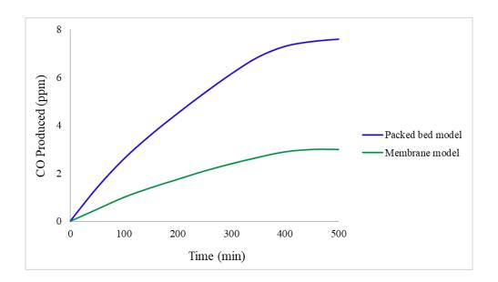
**Figure 3.** CO generated during reaction for the packed bed and membrane microreactors. Study performed at an inlet flow of 0.05 ml/min, reaction temperature of 30 °C, pressure 1 bar, and Pd/C catalyst.
