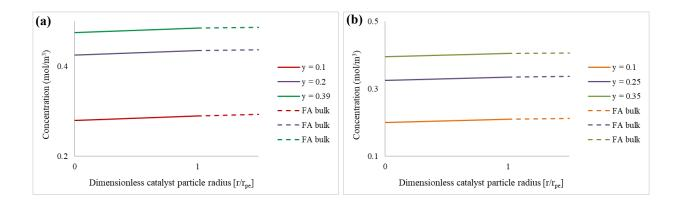
**Figure 7.** Formic acid concentration profiles within the catalyst particles and in the bulk fluid at x = 1.25 cm, using (a) coated wall; and (b) membrane microreactors. Study performed at an inlet flow of 0.05 ml/min, reaction temperature of 30 °C, pressure 1 bar, and Pd/C catalyst
