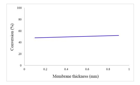
**Figure 9.** Influence of membrane thickness on the formic acid conversion. Study performed at an inlet flow of 0.05 ml/min, reaction temperature of 30 °C, pressure 1 bar, and Pd/C catalyst.
