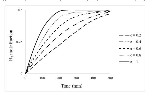
**Figure 10.** Mole fraction of hydrogen produced with time for varying catalyst coating thicknesses in the coated wall microreactor. Study performed at an inlet flow of 0.05 ml/min, reaction temperature of 30 °C, pressure 1 bar, and Pd/C catalyst.
