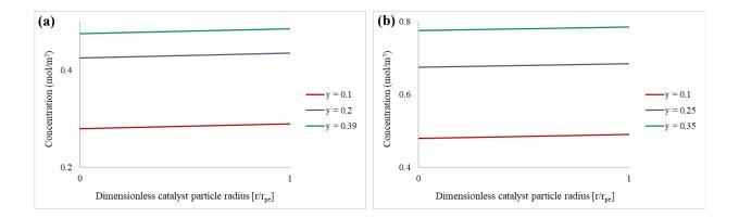
**Figure 6.** Formic acid concentration profiles within the catalyst particles at x = 1.25 cm, for (a) coated wall microreactor; and (b) membrane microreactor. Study performed at an inlet flow of 0.05 ml/min, reaction temperature of 30 °C, pressure 1 bar, and Pd/C catalyst.
