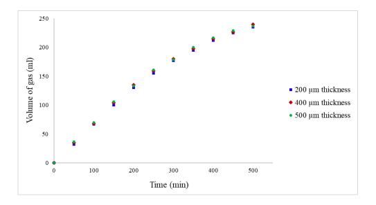
**Figure 8.** Influence of catalyst coating thickness on the volume of gas generated, with respect to time, in the coated wall microreactor. Study performed at an inlet flow of 0.05 ml/min, reaction temperature of 30 °C, pressure 1 bar, and Pd/C catalyst.
