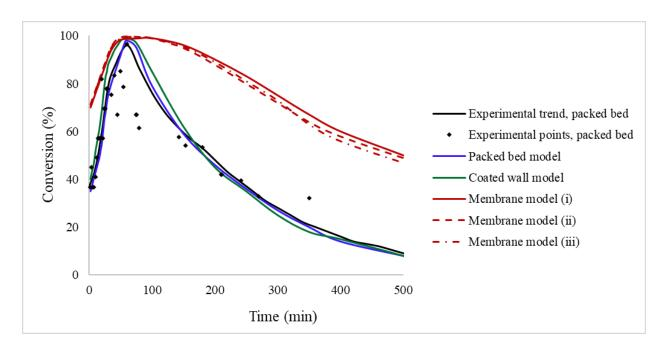
**Figure 2.** Experimental and CFD modelling results representing the conversion of formic acid against reaction time. Study performed at an inlet flow of 0.05 ml/min, reaction temperature of 30 °C, pressure 1 bar and Pd/C catalyst.
