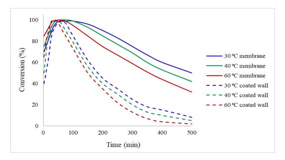
**Figure 4.** Impacts of temperature on the formic acid conversion using coated wall and membrane microreactors. Study performed at an inlet flow of 0.05 ml/min, reaction temperature of 30 °C, pressure 1 bar, and Pd/C catalyst.
