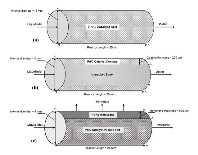
**Figure 1.** Representation of the (a) fixed bed; (b) coated wall; and (c) membrane microreactors developed for the CFD modelling study.
