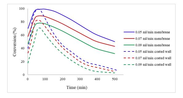
**Figure 5.** Formic acid inlet liquid flow against the formic acid conversion using coated wall and membrane microreactors. Study performed at a reaction temperature of 30 °C, pressure 1 bar, and Pd/C catalyst.
