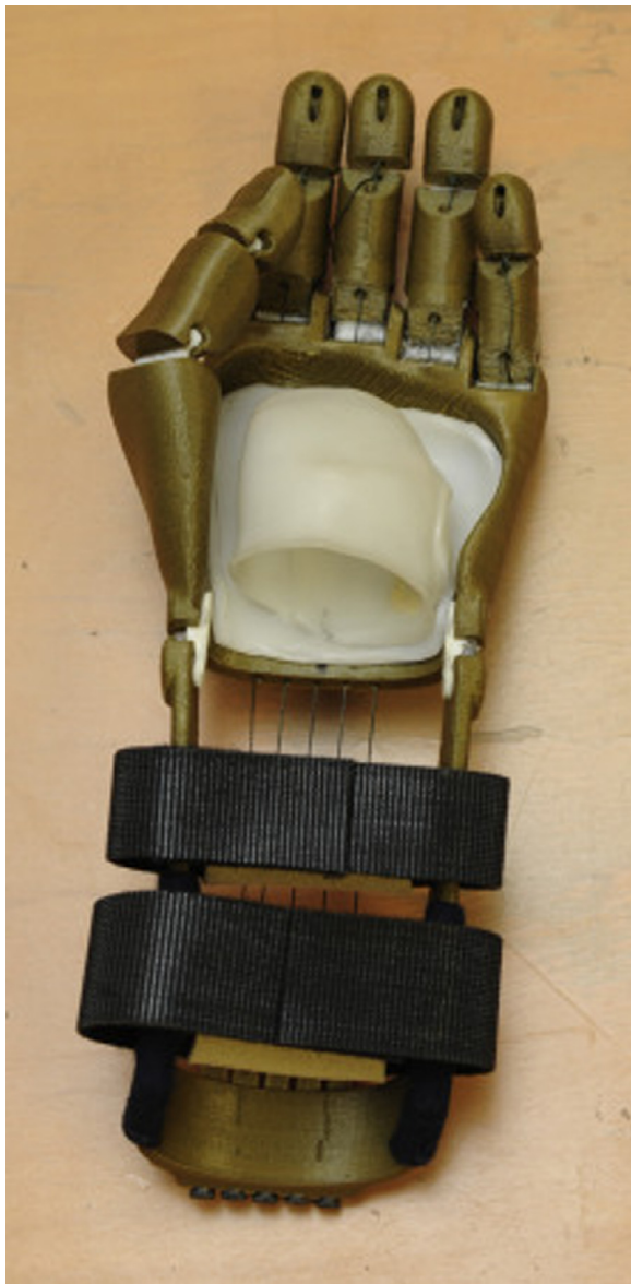
Fig. 2b – Image of 3D printed hand prosthesis. Permission granted from Fig. 5 of. 10
