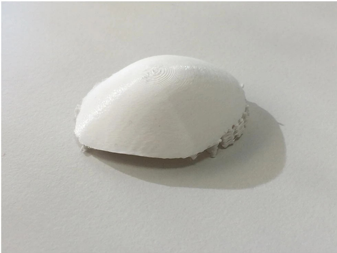
Fig. 7c – Image of a 3D printed scleral cover shell prosthesis using polylactic acid (PLA). Permission granted from Fig. 5 of. 66
