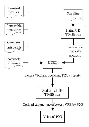
Fig. 2. Schematic representation of the soft-linking methodology.
