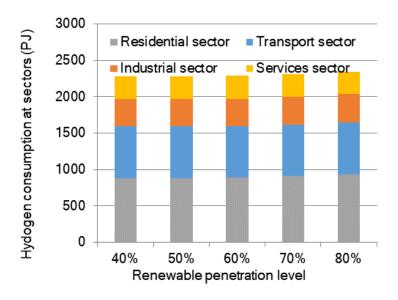
Fig. 5. Hydrogen consumption by sectors as identified by UK TIMES in 2050 under different assumption of renewable penetration levels.
