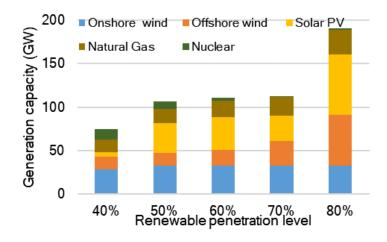
Fig. 4. Electricity generation portfolio identified by UK TIMES in 2050 under different assumption of renewable penetration levels.
