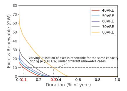
Fig. 8. Duration curve of hydrogen production from P2G under different renewable penetration levels..
