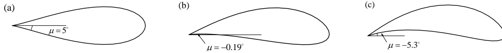
Fig. 6. The foil shape ( \xi_c = 0.1 , \tau = 10^\circ ): (a) \eta_c = 0(\mu = 5^\circ) , (b) \eta_c = 0.1(\mu = -0.15^\circ) , (c) \eta_c = 0.2(\mu = -5.3^\circ)
