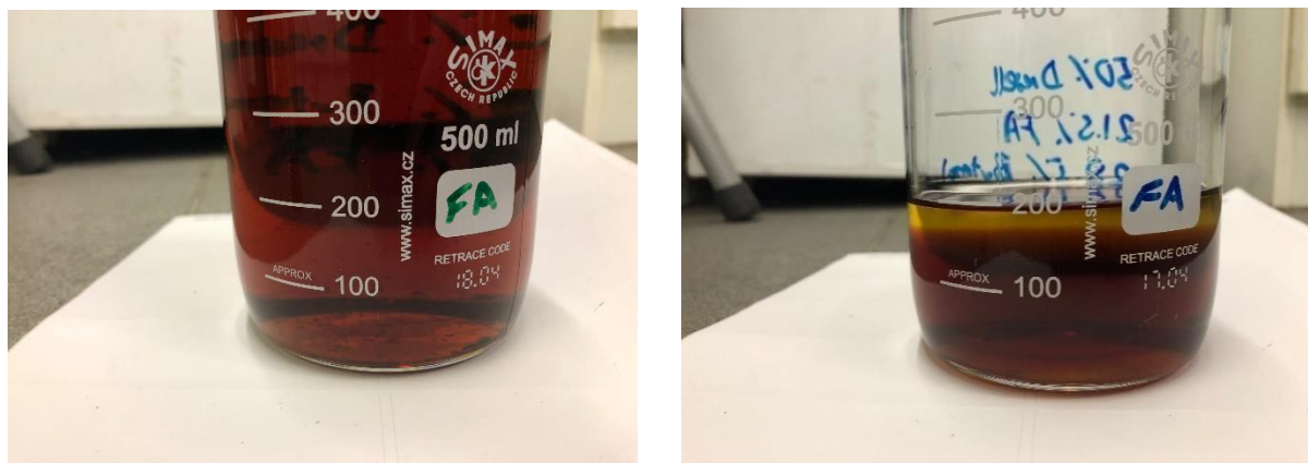
Figure 4.1: Comparison of 50:50 furfuryl alcohol blend with diesel having formed a homogenous mixture (a) and a visibly separated mixture (b)
