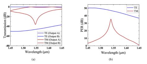
Fig. 7. (a) The transmission and (b) the PER versus wavelength.
