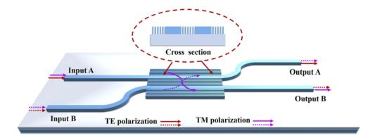
Fig. 1. The 3D schematic view of the AM PBS.
