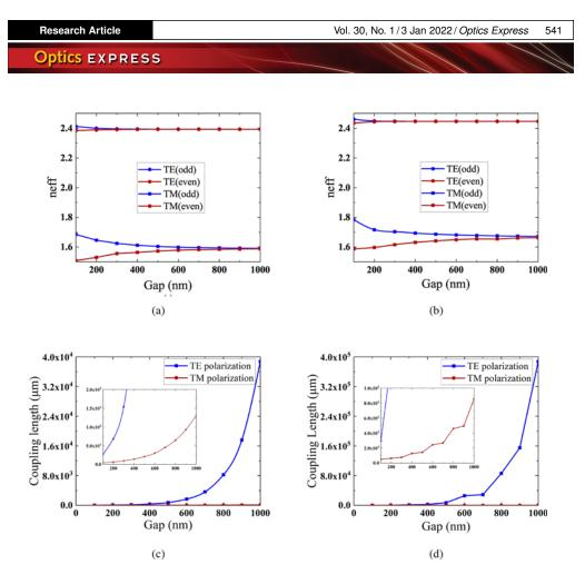
**Fig. 3.** The effective refractive index versus the gap for (a) normal PBS and (b) AM PBS. The coupling length versus the gap for (c) normal PBS and (d) AM PBS.
