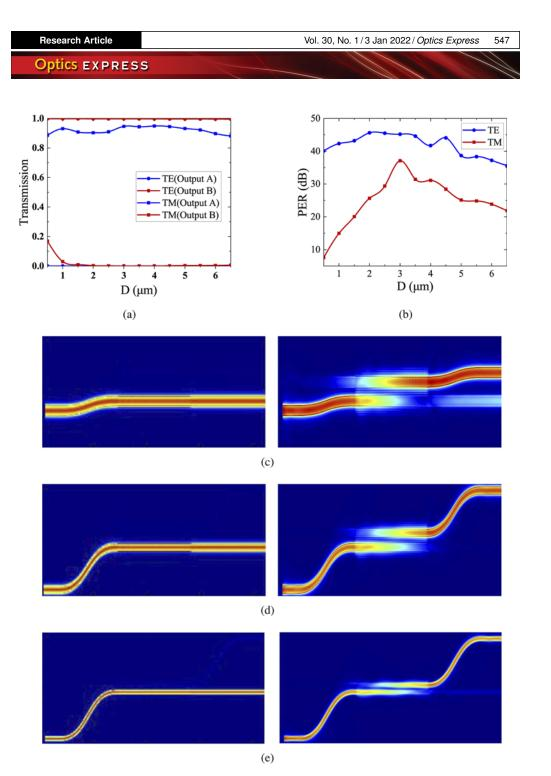
**Fig. 8.** (a) Simulated transmittance and (b) PER versus with the vertical distance of the S-bend waveguides, with incident light from Input B. Electric field distribution along the PBS with the vertical distance of the S-bend waveguides of (c) 0.5  $\mu$ m, (d) 3  $\mu$ m, and (e) 6.5  $\mu$ m.
