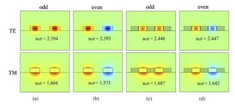
**Fig. 2.** The electric field distribution of TE and TM modes in the coupling waveguides with and without AM structures.
