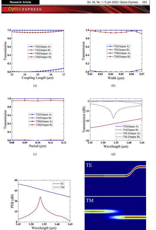
**Fig. 4.** The transmission versus (a) coupling length, (b) strip width, (c) period of the AM PBS. (d) The transmission and (e) the PER versus wavelength. (f) The optical energy distribution of the optimized AM PBS.
