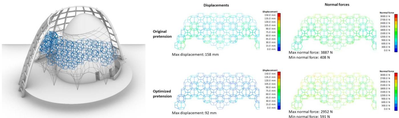
Figure 1. The distance to the target net under live loads is minimized by optimizing the tension in the outer cables.
