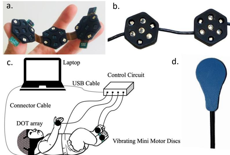
Fig. 1. ANIMATE v1 triple-hexagonal module design (a). ANIMATE v2 connected hexagonal modules (b). Infant DOT sensorimotor imaging arrangement (c). Silicone encapsulation of the vibrating DC micro motor (d).
