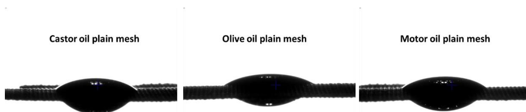
Supplementary figure (S6.6). The contact angles of the oil on the plain mesh are shown. All the oils wet the stainless-steel well and pass through, each having a similar contact angle.
