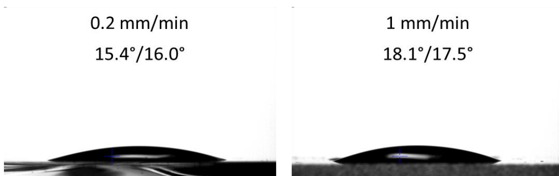
Figure 5.4. The average wetting of the ordered macroporous monolayer inverse coatings is shown. The samples were more hydrophilic than the glass microscope slide substrates.
