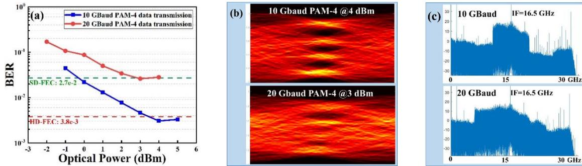
Fig. 2. (a) The BER performance for the 10- and 20 GBaud PAM-4 signals after wireless transmission. (b) Eye diagrams of 10 GBaud PAM-4 signal at 4 dBm optical power and 20 GBaud at 3 dBm. (c) The electrical spectra of the 10- and 20 GBaud PAM-4 signals after the down conversion.
