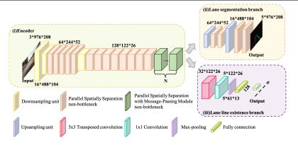
Figure 3: Overall architecture of the proposed PSSNet.
