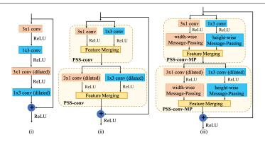
Figure 2: Three different residual layer modules: (i) the non-bottleneck-1D module in ERFNet; (ii) the PSS-nbt module; (iii) the PSS-nbt-MP module.
