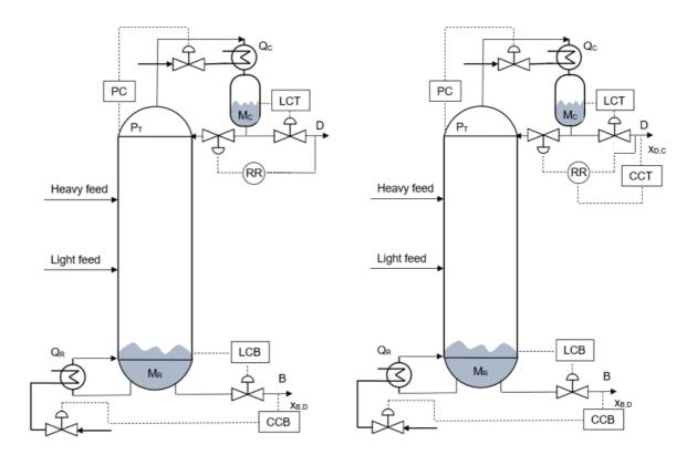
Figure 2: V-only (left) and LV (right) control configurations.
