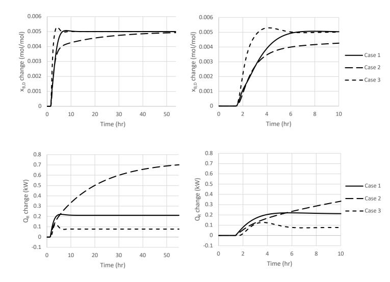
Figure 17: Control performance of MPC for all case studies towards bottom product purity set point change. Bottom product purity response and reboiler duty are presented from top to bottom, respectively. Left figures show full time scale whilst figures on the right focus on initial responses. Disturbance introduced at t=1.4 hrs.
