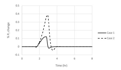
Figure 15: Control responses to feed composition disturbance using optimised tuning parameters as shown in Table 5 (Case study 1 and Case study 2, LV control). Disturbance introduced at t=1.4 hrs.
