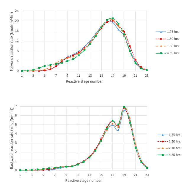
Figure 5: Reaction rate (forward-top and backward-bottom) change due to the introduction of feed B flow rate disturbance (5% increase). Disturbance introduced at t=1.4 hrs. Stages 1 (condenser) and 25 (reboiler) are not considered reactive, therefore reactive stages only are shown. (Case study 2, V-only control).
