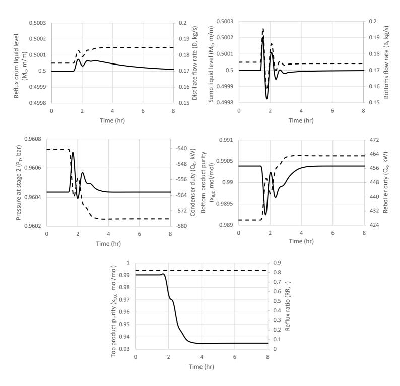
Figure 3: Closed-loop responses for feed B flow rate disturbance (5% increase). Disturbance introduced at t=1.4 hrs. Left axis is controlled variable (solid line) and right axis is manipulated variable (dashed line). (Case study 2, V-only control).
