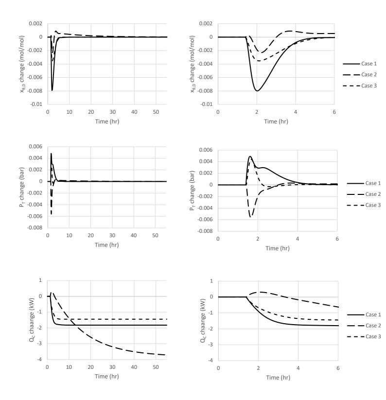
Figure 18: Control performance of MPC for all case studies towards feed B flow rate disturbance. Bottom product purity, pressure and condenser duty are presented from top to bottom, respectively. Left figures show full time scale whilst figures on the right focus on initial responses. Disturbance introduced at t=1.4 hrs.
