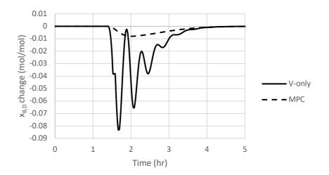
Figure 16: Difference in bottom product purity response to feed flow rate disturbance using conventional V-only control (solid line) and linear MPC (dashed line) for Case study 1. Disturbance introduced at t=1.4 hrs.
