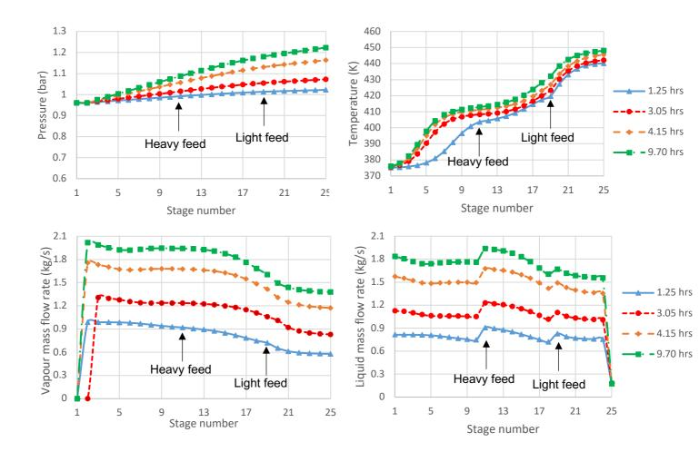
Figure 8: Pressure (top, left), temperature (top, right), vapour mass flow rate (bottom, left) and liquid mass flow rate (bottom, right) change due to the introduction of feed B flow rate disturbance (5% increase). Disturbance introduced at t=1.4 hrs. (Case study 2, LV control).
