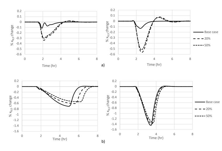
Figure 13: Bottom product purity response to feed flow rate (left) and feed composition (right) disturbance for increased tray liquid holdup. Disturbance introduced at t=1.4 hrs. (Case study 2, V-only (a) and LV (b) control).
