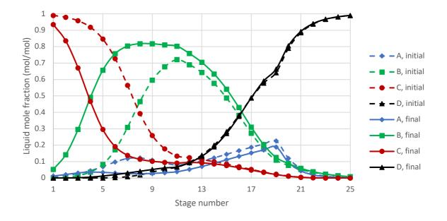
Figure 6: Composition profiles change due to feed B flow rate disturbance (5% increase). Initial: steady state value before the introduction of the disturbance, Final: indicates the new steady state value after the disturbance has settled in the column. (Case study 2, V-only control).
