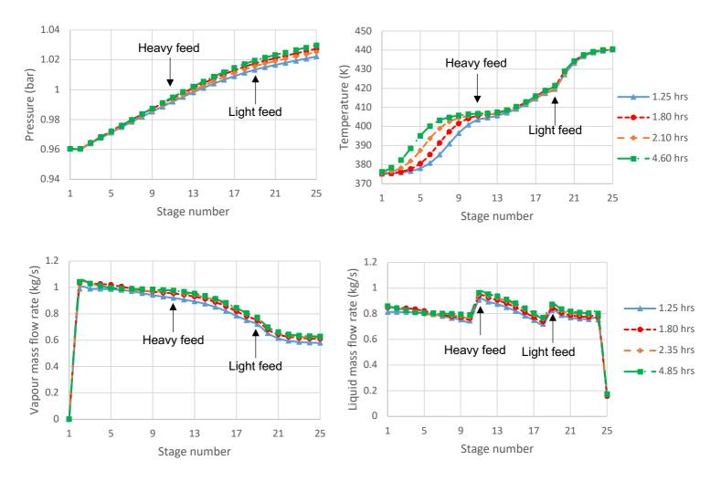
Figure 4: Pressure (top, left), temperature (top, right), vapour mass flow rate (bottom, left) and liquid mass flow rate (bottom, right) change due to the introduction of feed B flow rate disturbance (5% increase). Disturbance introduced at t=1.4 hrs. (Case study 2, V-only control).
