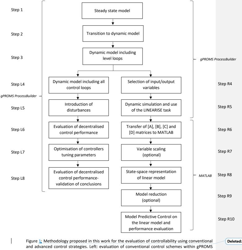
and advanced control strategies. Left: evaluation of conventional control schemes within gPROMS ProcessBuilder, Right: evaluation of Model Predictive Control on a linearised model using both gPROMS ProcessBuilder and MATLAB. The methodology should be repeated several times based on the purpose of the investigation as explained in section 2.
