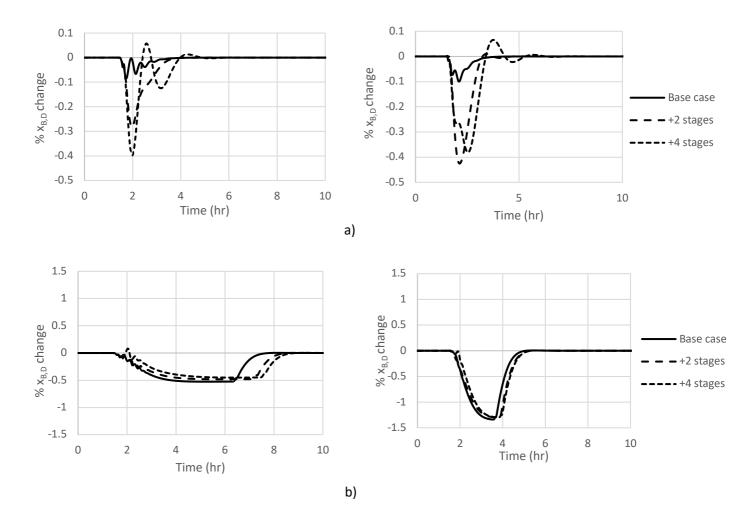
Figure 12: Bottom product purity response to feed flow rate (left) and feed composition (right) disturbance for additional number of stages of reactive column. Disturbance introduced at t=1.4 hrs. (Case study 1, a) V-only control; b) LV control).
