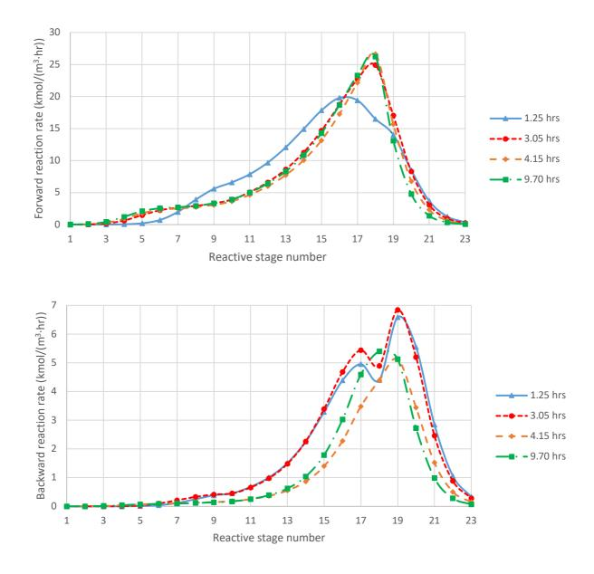
Figure 9: Reaction rate (forward-top and backward-bottom) change due to the introduction of feed B flow rate disturbance (5% increase). Disturbance introduced at t=1.4 hrs.
