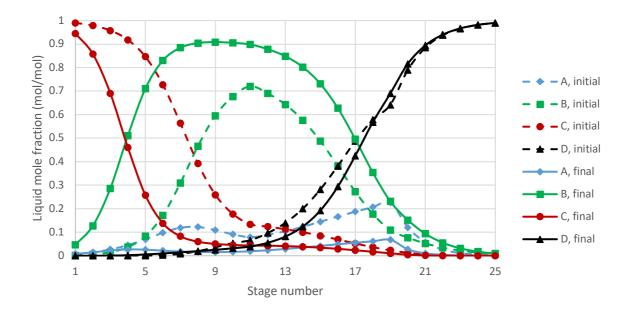
Figure 10: Composition profiles change due to feed B flow rate disturbance (5% increase). Initial: steady state value before the introduction of the disturbance, Final: indicates the new steady state value after the disturbance has settled in the column. (Case study 2, LV control).
