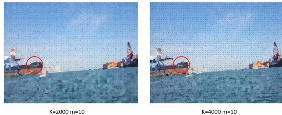
Figure 8. For m = 10 , iteration=10, the output of the SLIC algorithm module for K = 2000 and K = 4000 .
