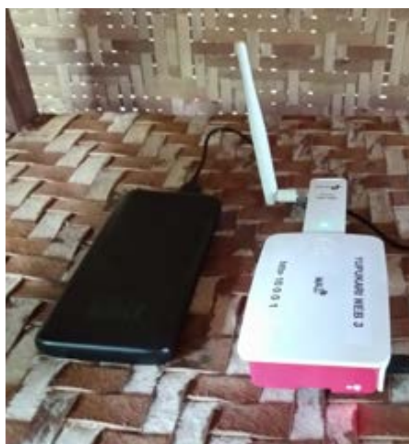
Battery powered Raspberry Pi: community story sharing in a remote village in Guyana
